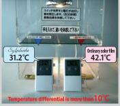
Sylphide is high functional film to provide clear visibility together with comfortable and classy atmosphere by the selection of shade efficiency which can keep heat down by filtering infrared rays more than 90%.
